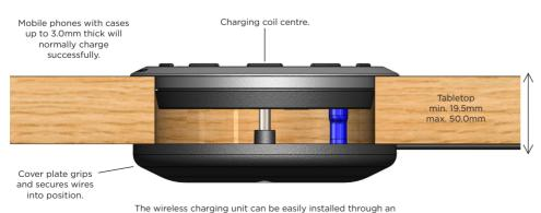
Ø80.0mm hole in any flat surface. Cables are secured by the retaining plates completing the installation.
