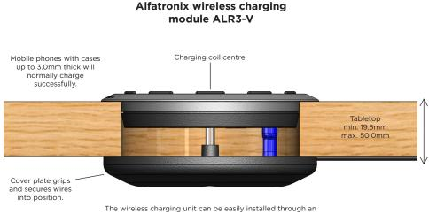
The wireless charging unit can be easily installed through an Ø80.0mm hole in any flat surface. Cables are secured by the retaining plates completing the installation.
